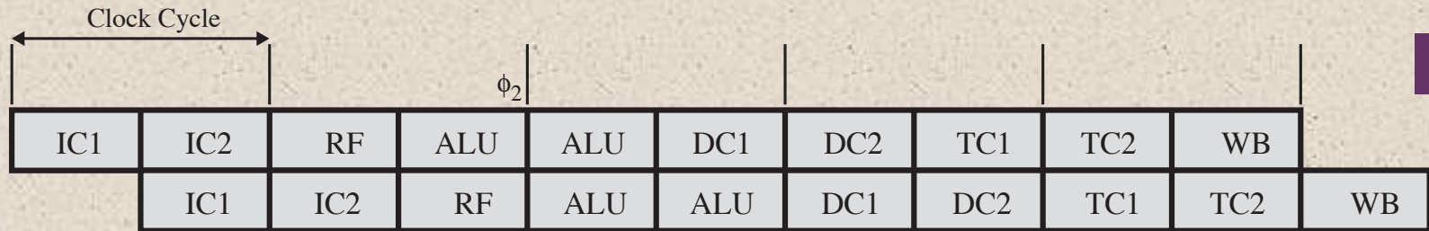
(a) Superpipelined implementation of the optimized R3000 pipeline
