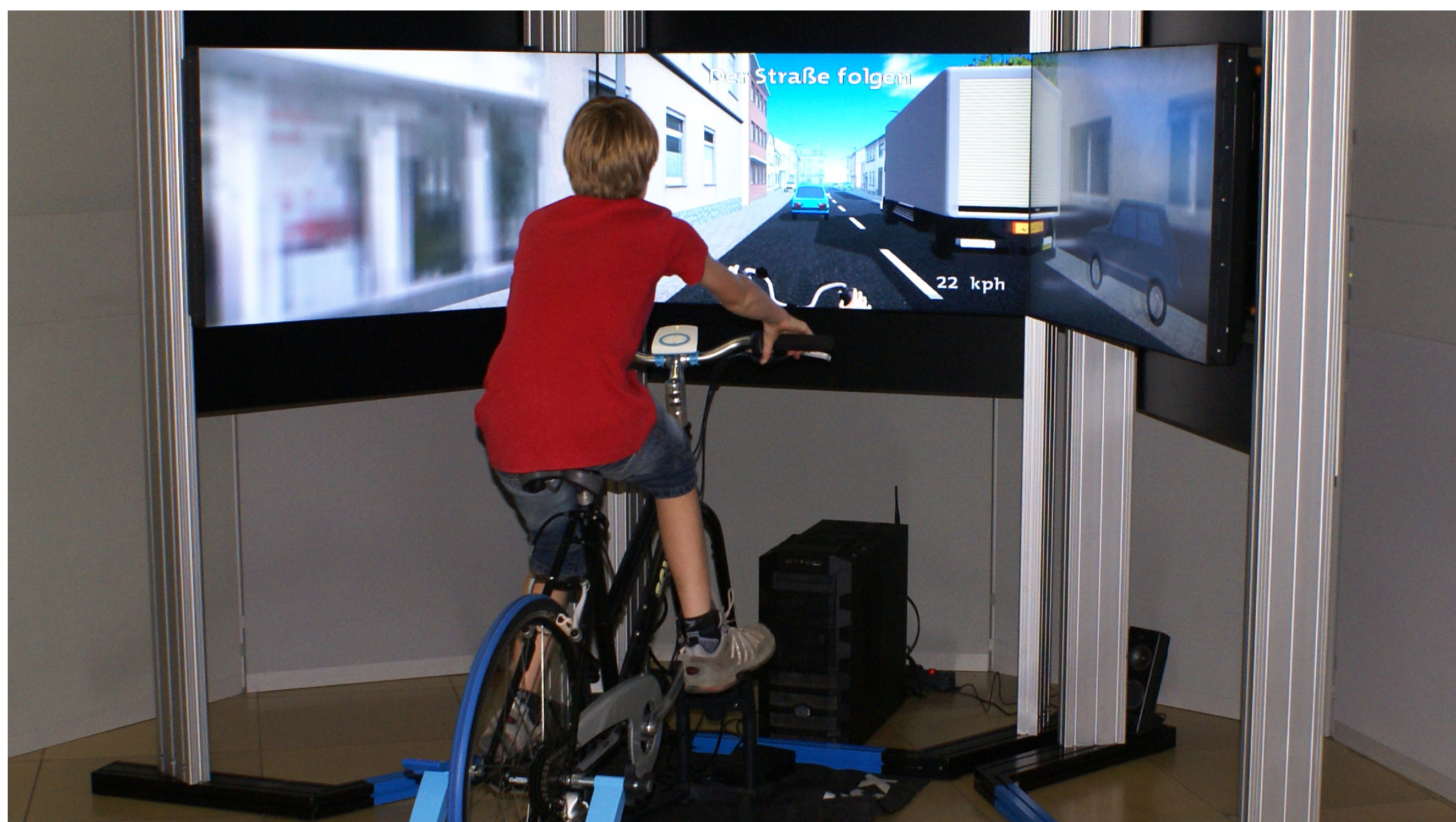
Figure 1. The FIVIS simulator with its compact three-screen immersive visualization system.
