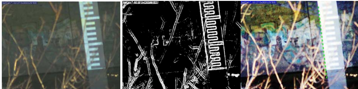
Figure 2: On the left is the original image showing water on the pier marker on Jan. 13, 2008. The middle image is the result of processing the original with an edge detection filter. The right image is a histogram equalized version of the original, and has a green line on the left edge of the pier marker indicating the detected edge location.
